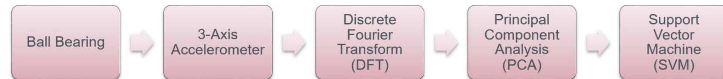
Figure 3. Example of a FDD process for a system with a cracked ball bearing.
