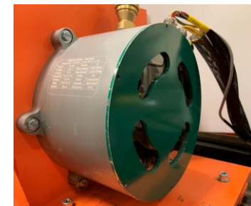
Fig. 2. Scaled-down prototype of proposed PMSM.
